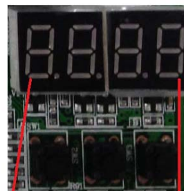
E shows failure occur
