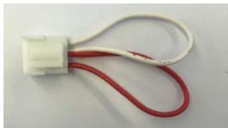
Figure 1 short wiring
